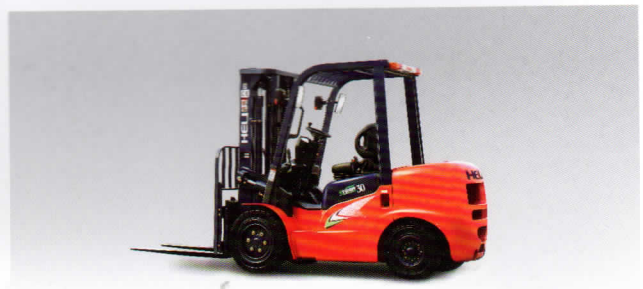
G Series, diesel, Pneumatic CPCD10-35 2,000 - 7,000 lbs
