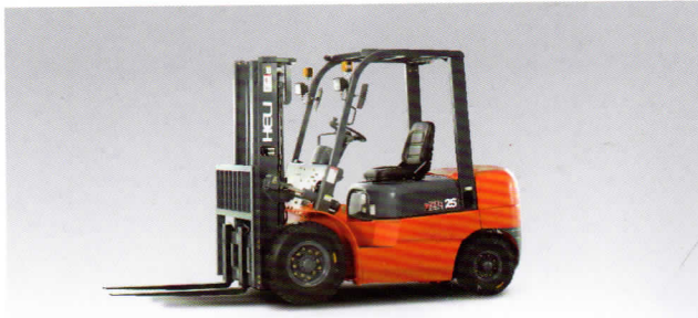
Dieisel,Pneumatic Forklift CPCD 10-35 2,000-7,000lbs.
