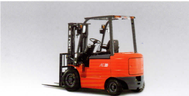
48V AC 4-Wheel Electric forklift CPD10-25 2000-5000 lbs.
