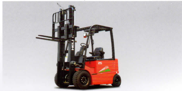
G Series 48v 4-Wheel Electric Forklift CPD10-25G 2,000-5,000 lbs.
