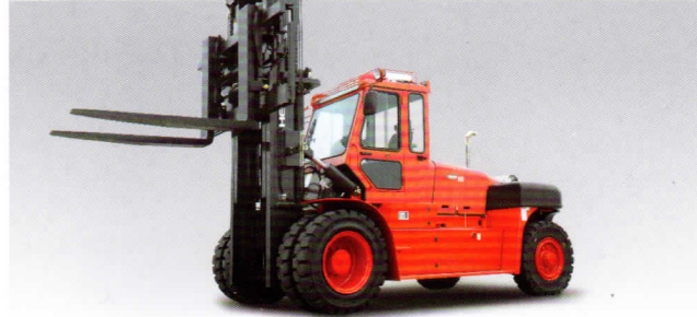
Diesel, Pneumatic Forklift CPCD120-135 26,500 - 30,000 lbs
